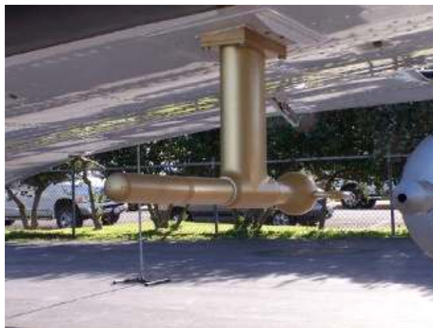
Figure 1: AIMMS-20 Under-Wing Air Data Probe Installation
