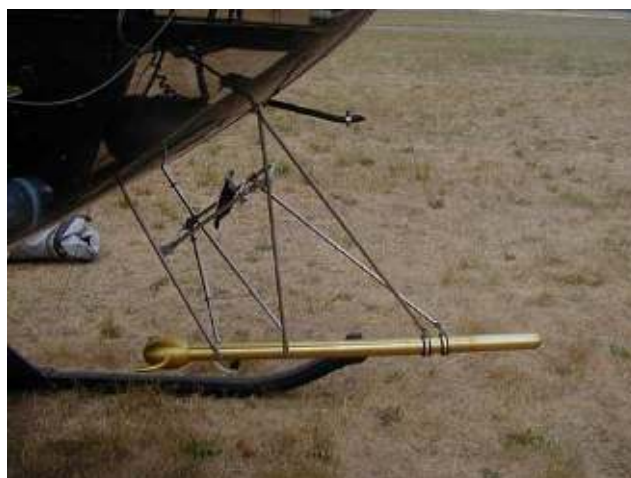
Figure 2: AIMMS-20 Sting-Mount Air Data Probe Installation
